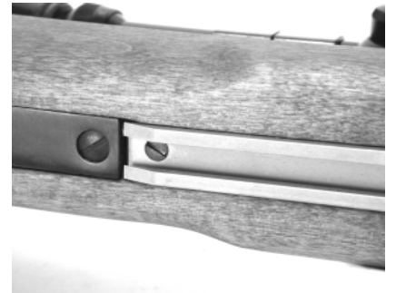
The forend rail allowed the shooter to move his front support hand and sling to nearly any position.
