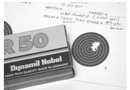
This group, shot at 50 yards with RWS R50 ammunition, shows how accurate the CM12 can be. One reason: The barrel and action float away from the wooden stock.
