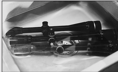
Above: To check for fogging, we dunked each scope in a warm-water bath for 10 minutes, then cooled the scope in a freezer for 30 minutes.
