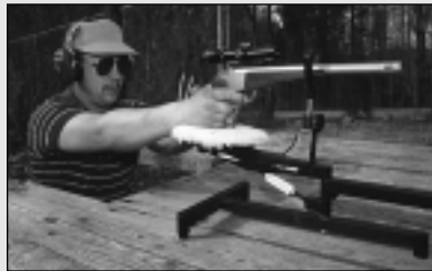
Above: The .45-70 Government is another good Contender cartridge, especially with a hard-cast bullet from the RCBS 45-458-FN mold. Fifty grains of IMR 3031 or 48 grains of H-332 powder with a CCI LR primer will push the projectile to about 1,400 fps.
