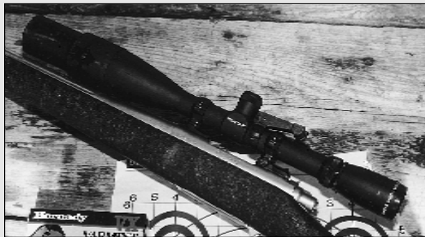
Above: We equipped each rifle with a Pentax 6-24 MC AO Lightseeker scope mounted in Millett rings and bases. By equipping all four rifles with the same riflescope model, we were able to eliminate one variable.
