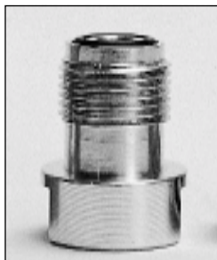
Above and below left: To get the Morini nipple to work, we had to machine metal off the connector (arrows) to allow the DIN nipple to seat in the valve. Below right: The Anschütz nipple also needed relief, and we machined flat sides on the nipple to make tightening and loosening the nipple easier.
