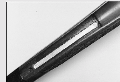
Above: To make the forend stiffer and more resistant to flexing, we routed a channel in the forend and bedded in a high-strength aluminum rod into the channel.
