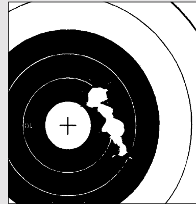
Above: We were able to fire cold-barrel \frac{5}{8} -inch groups with factory ammo once the barrel had been scrubbed.
