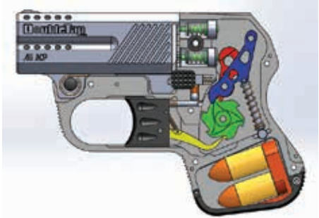
This company schematic shows the guts of the DoubleTap pistol. The two rounds in the grip are extras.
