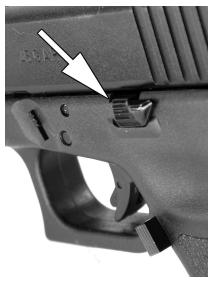
Left: The slide release was snag free but easier to engage than the original design. We didn't really need to add an extended magazine release. It stuck out too much when added to the slim frame of the model 38. It didn't cause the magazine to be released unintentionally, but the standard size button is a better choice.
