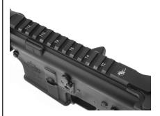
Clearly numbering the notches in the Picatinny rail was very helpful for mounting (and remounting) the scope with proper eye relief.
