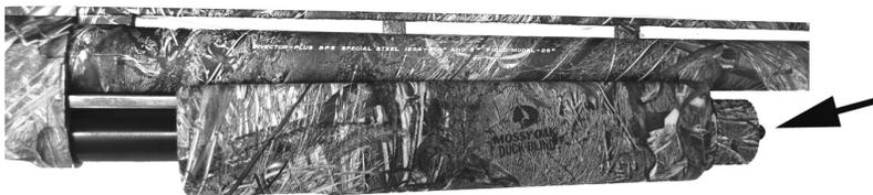
A good fit for all the members of our test team, only minor adjustments were required for us to get into pump-action mode of shooting. Note that the end of the magazine cap is where the sling attachment is located.
