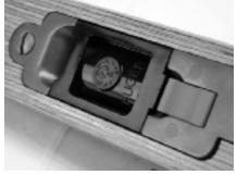
when ordering. The flush-fitting 9-round magazine was helpful in maintaining a uniform surface for shooting from support.
