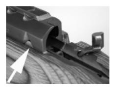
The three-position safety allowed for removing the bolt with the trigger locked. The bolt release was the slim button shown inside the relief on the left side of the action.
