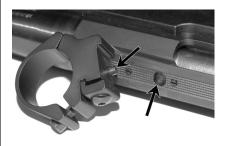
The arrows point to a pin on the supplied front ring of the Tikka T3, and to a hole in the top of the action which accepts the pin. The pin fits loosely, but when moved to the front, this prevents the scope from kicking forward on recoil. The rear ring didn't have the pin. Note the easy, rugged, Allenheaded mounting system, and the notched rail in the top of the action to which the ring clamps.
