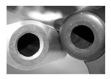
The barrels on both Ruger SP101s were properly crowned, as shown by the shape of the SP101's muzzle on the left. This simple finishing touch helped prevent fliers, such as the ones that marred the accuracy of the Heritage Rough Rider, the muzzle of which is
