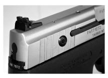
The rear sight was adjustable for windage only. We liked the way it played "peek-a-boo" with the white dot on the front sight. The key-operated lock was on the slide, and the extractor had a chamber-loaded indicator.
