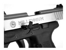
All levers were on the left side of the pistol. From the rear forward are the thumb safety, slide release, and the slide-stop pin, shown ready for takedown.
