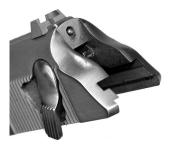
Left in the down position, the slidemounted decocker deactivated the trigger. The small pin located below the rear sight (arrow) was the chamberloaded indicator. The firing pin is out of sight, recessed from the rear of the
