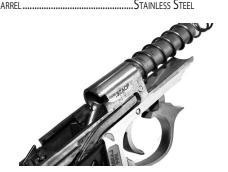
Blowback design meant that the barrel was fixed in place. Note the stout recoil spring surrounding the barrel.
