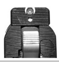
Right: We found a major problem with the rear sight in that it was razor-sharp. The customer specified this type sight, which he ended up not liking. It's easy to cycle the slide with one hand, using a sight of this type to catch on any suitable surface.
