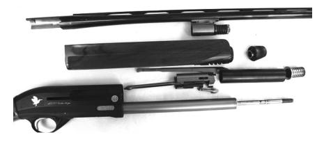
Because of its gas-operated system, the Beretta is more complicated and becomes fouled quicker than the two Benelli shotguns.
