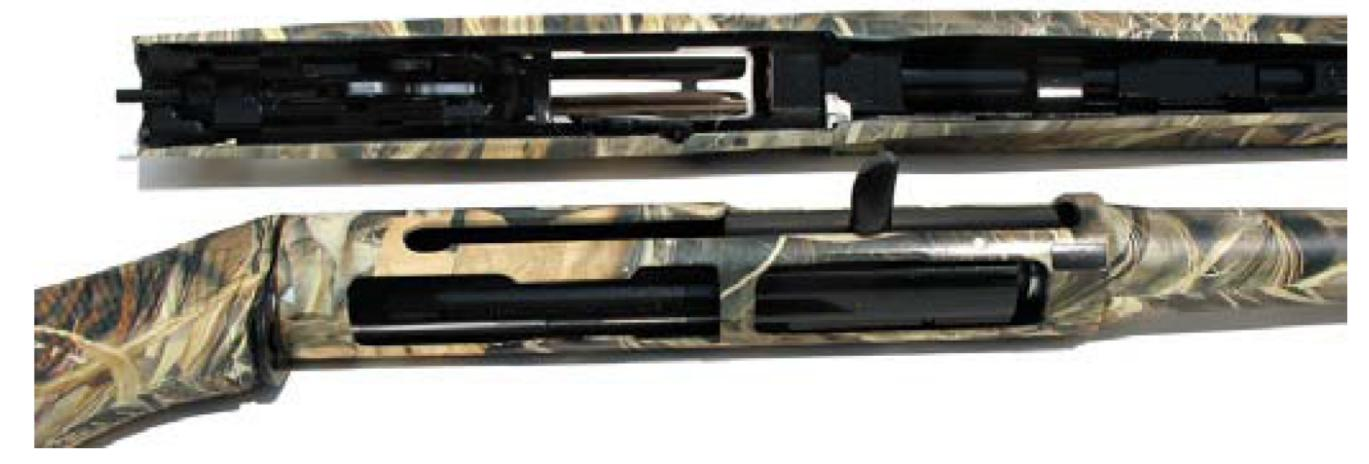
A push of the forearm button, a twist of its knob, and the Vinci "lower" comes free in seconds. If you'd like to go farther, the buttstock comes off with a 90-degree twist. We have no idea what practicality fast buttstock removal might have, but we did appreciate the quick "no tools" access to the trigger group for periodic cleaning.
