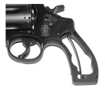
Replacing the too-thick rubber unit with wood or other panels that expose the back strap would shorten the trigger span and make it easier to reach that trigger for DA use.
