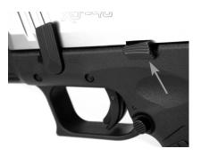
The company website offers several pages touting new features but missed the new slide release (arrow). We liked its accessibility much better than the original. The trim contour of the slide negated the need for a pass-through slot to accommodate the slide latch, shown in the release position.
