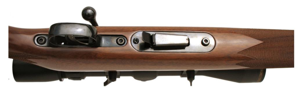
Above: The Savage had excellent wood-to-metal fit, but its magazine, seen protruding here, was a drawback to our testers. At right is the Ruger. The flush surface of the rotary Ruger magazine gave the
