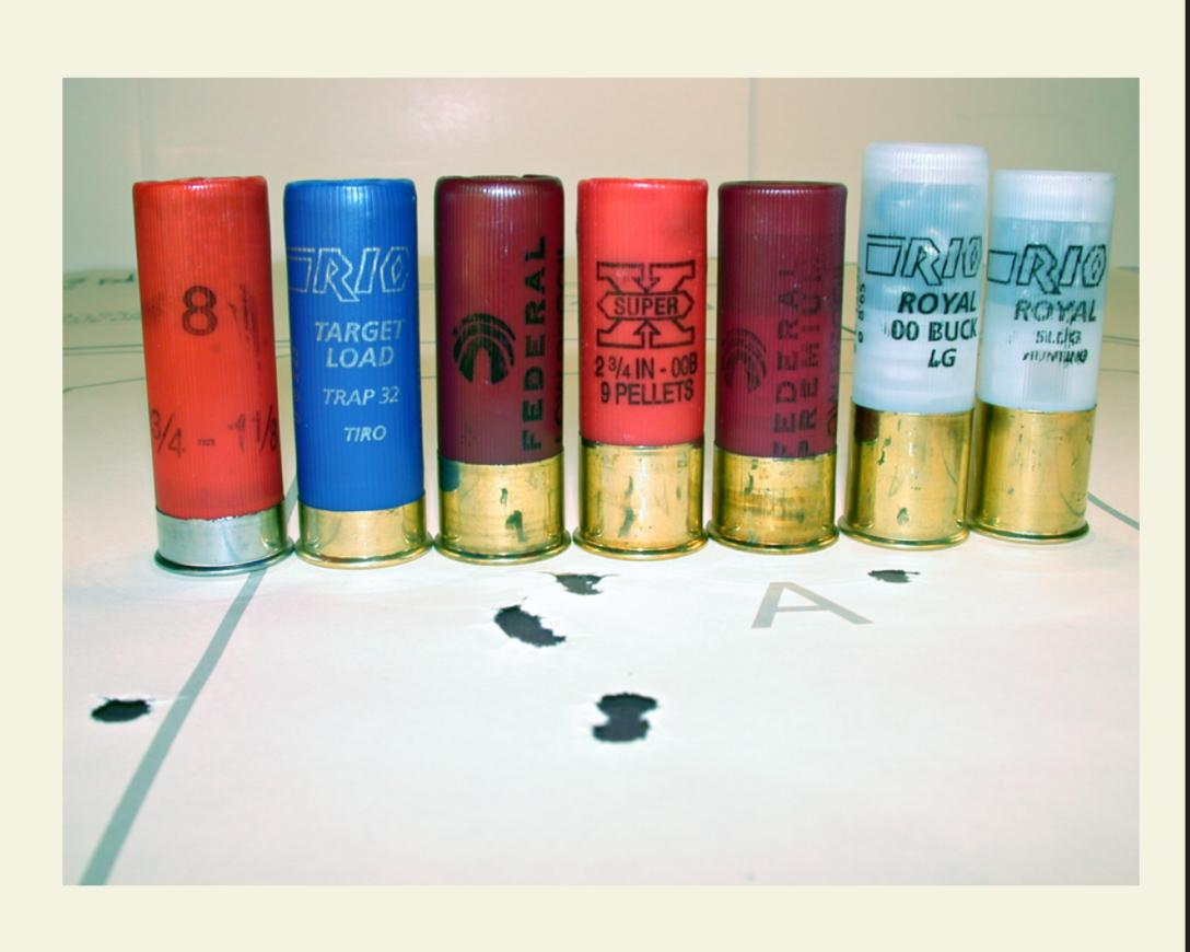
all Federal Low Recoil Rifled Slug No. PB127LRS. The last two cartridges are Rio's Royal buckshot and Royal slug. These two rounds were deleted from the test when it was determined that they would chamber in our test guns but not cycle from either magazine. This was our only incident of malfunction with either shotgun. The pattern shown was produced by nine pellets of Federal buckshot fired by the CZ USA 712 Utility from a distance of 10 yards with the Cylinder choke-tube installed.
