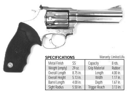
All eight of the Model 941's chambers were tight enough to make extraction very hard with most of the ammunition we tried. It was the only revolver tested here with a full-length barrel underlug.
