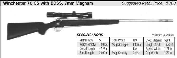
The Model 70 Classic Stainless has a pre-'64 bolt with a claw-type extractor that provides controlled feeding. The downside is that the bolt won't close if a round is inserted manually into the chamber.
