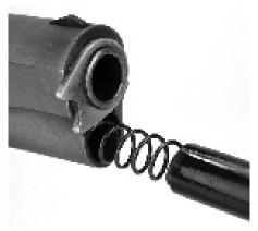
Above: We could turn the bushing by hand, so no tools were necessary to remove the top end. Note the low front sight. Today's low-mount front sights are more visible.
