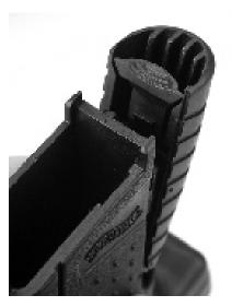
The backstrap was held in place by a leaf spring. Removing the backstrap also disabled the pistol. The release was shielded once the magazine was in place but one clumsy reload and you could end up dumping the backstrap. Also, once removed, this small part would be easy to lose.
