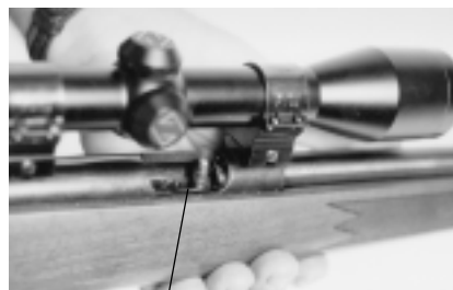
The Remington's clip protruded from the bottom of the gun, creating feeding problems when the left hand pushed the magazine upward.
