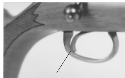
The Remington's trigger shoe had sharp edges at the bottom of the shoe.
