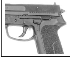
The polymer construction of the Sig Pro's frame dictated that its controls be designed differently than Sig's standard P-series pistols. However, the location and operation of the controls are the same.
