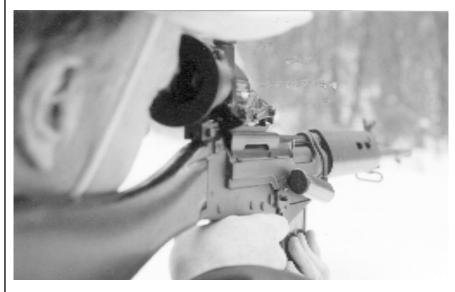
The L1A1 shines in any weather with its SUIT scope. The SUIT, or Trilux, or L2A2 scope is today sold without the original green radiating element that illuminated the reticle. However, a battery unit is available to light the inverted post red, for better visibility in marginal light. This efficient combination rated very close to the M1A in our tests. This one is built on the Entreprise receiver.
