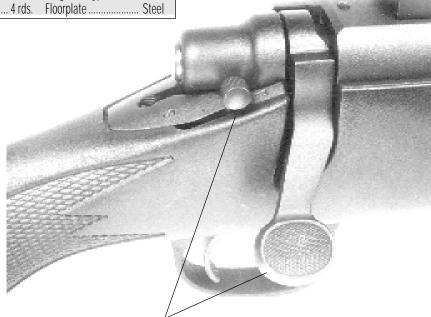
Like all Remington Model 700s, the ADL Synthetic's manual safety is a two-position lever behind the bolt on the right rear of the receiver. The bolt knob is flattened.
