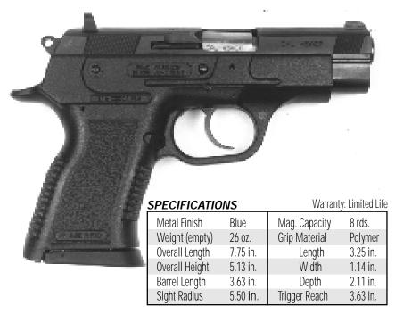
Our test gun's barrel and slide had a significant amount of play. It failed to feed numerous times with ball and hollow point ammunition. This pistol also had the longest trigger reach.
