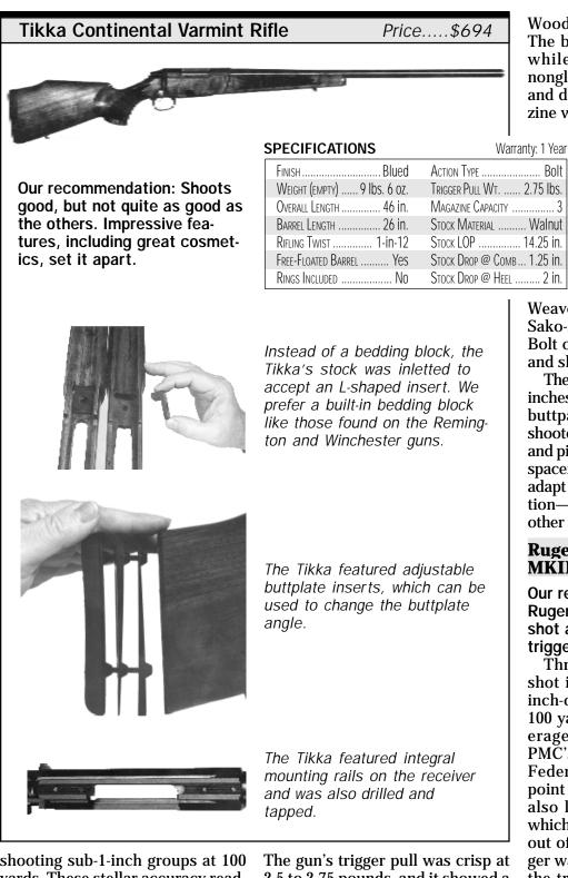
shooting sub-1-inch groups at 100 yards. These stellar accuracy readings derive from the gun's heavy barrel, the muzzle OD of which measured 0.770 inch at the crown, with a slight taper on the 26-inch free-floated barrel. An inspection of the gun's bore with a Hawkeye 17inch borescope showed no anomalies that would hinder accuracy. The gun's trigger pull was crisp at 2.5 to 2.75 pounds, and it showed a little creep. The trigger could be adjusted for pressure only.
