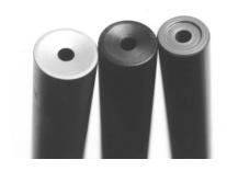
At 10 pounds 4 ounces, this was the heaviest of the test guns. A 0.87-inch-thick muzzle diameter (far left) accounted for the extra weight. The Remington barrel is shown center, and the Ruger is at right.
