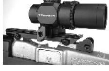
The top strap of the Ruger was cut for proprietary rings, and that is best for mounting a scope. But if you want to mount a cutting-edge tactical scope, such as the Leupold Prismatic shown here, we recommend installing the \$50 Weigand Combat mount from brownells.com.
