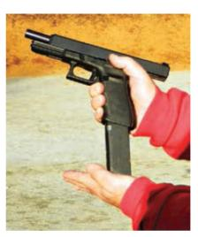
The Glock 41 allowed a trained shooter to get back in operation very quickly by using the welldesigned magazine release and tapered magazine.
