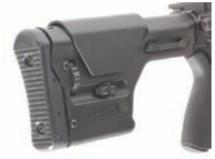
The Enidine Hydraulic Buffer is housed in the excellent PRS stock. The buffer makes the recoil pulse noticeably softer and smoother when shooting heavier loads. However, the manufacturer warned that functionality might be affected with lighter loads. We never experienced function problems prior to shooting the Tulammo. The buffer is no longer offered, and it is easy to exchange the hydraulic buffer with a standard buffer if the shooter wishes.
