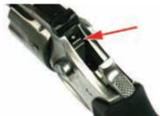
The hammer spur was coarsely checkered for a sure grip; note that the transfer bar just behind the firing pin will raise before it is hit by the hammer. Singleaction trigger pull was nice at 4.8 pounds.
