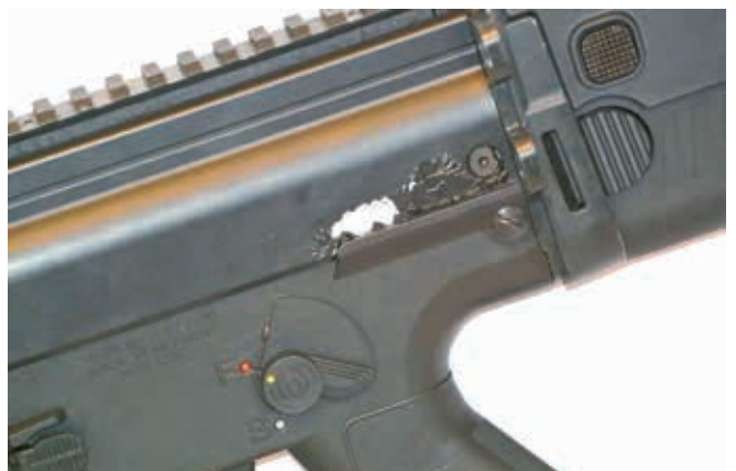
The ISSC MK22's finish quickly started to bubble and peel off in multiple locations.
